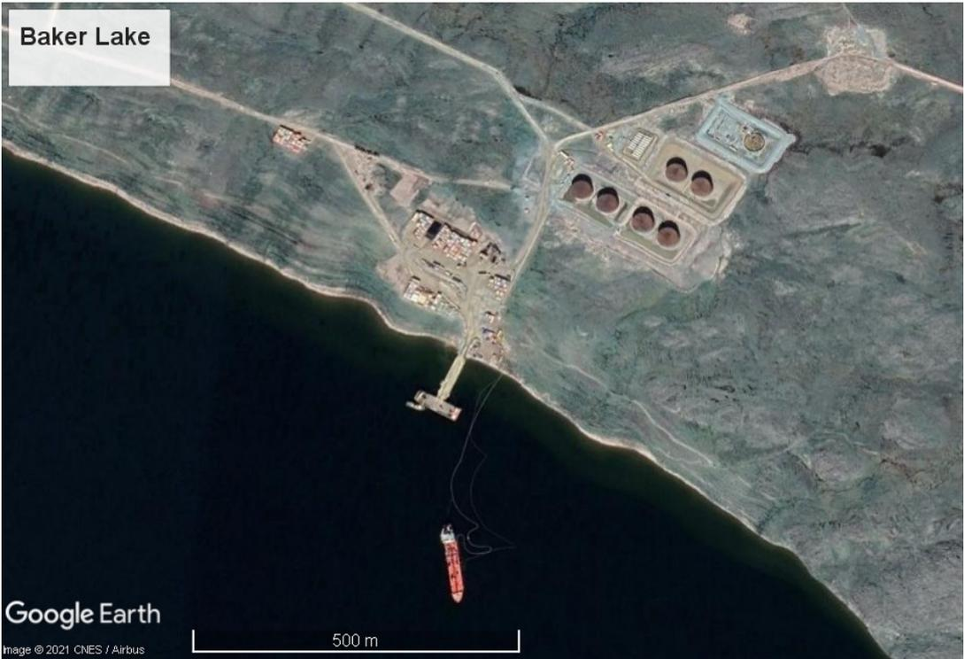
Note that the tanker is moored offshore while unloading fuel.
